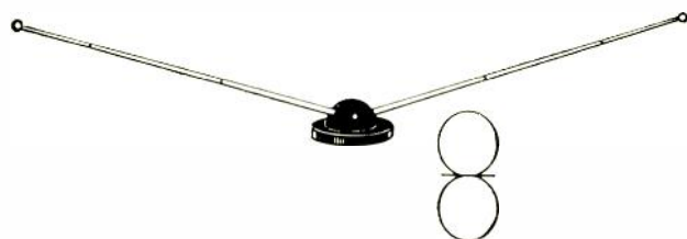
Figure 2. A TV rabbit-ears antenna is actually a half-wave dipole. "half-wave" meaning that it is tuned (by its dimensions) to half the wavelength it is designed to receive. At the center of the FM band, half a wavelength is equal to sixty inches.
