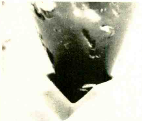
Figure 1 Two photomicrographs (taken with the scanning electron microscope) of a conventional 0.7-mil spherical-diamond stylus resting in a record groove that carries sine-wave signals at frequencies from 2,000 to 20,000 Hz recorded with vertical modulation. The same view is shown at two different magnifications (indicated by calibration marks).
