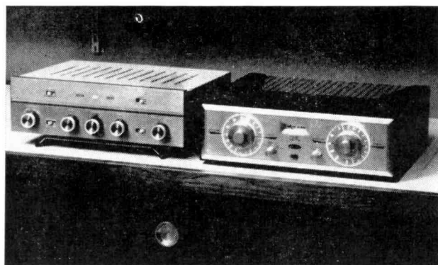
The Scott tuner shown with an early Bogen stereo amplifier had separate AM/FM tuning dials for reception of stereo broadcasts.
