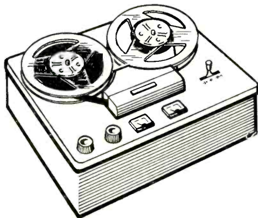
The tape deck will record and play back and may have a separate playback head that permits off-the-tape monitoring. Neither power amplifiers nor speakers are included.
