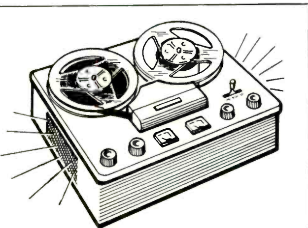
The full recorder includes a stereo amplifier with output power between 1 and 10 watts per channel, plus a pair of speakers either built-in or as part of the cover.
