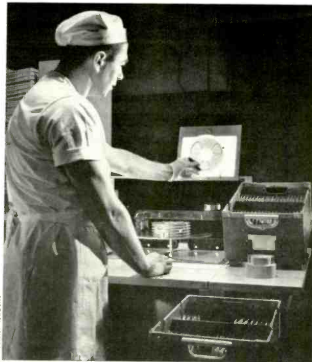
Each tape must be inspected for physical and magnetic defects.
