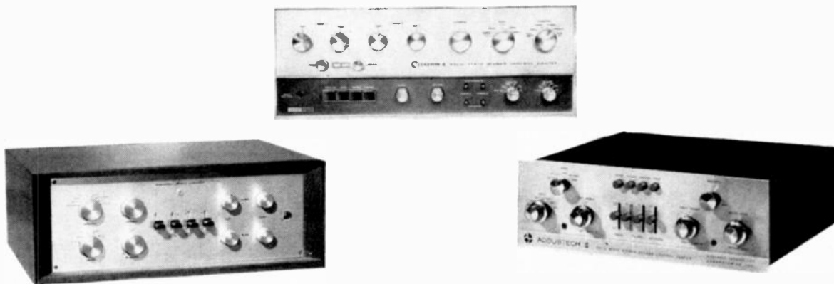
Three control-center stereo preamplifiers from the Ultimate Frontier group. Both the Citation A and the Acoustech II (center and right) are transistorized; the Marantz (left) employs tubes. All three are used with power amplifiers.
