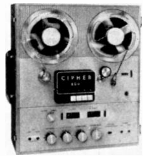
CIPHER 800 a professional 4-track stereo recorder with 3 hysteresis-synchronous motors and 3 heads; plug-in head assembly (2-track also available); no pressure pads, tape speeds 7\frac{1}{2} and 3\frac{3}{4} ips, solenoid controlled, 2 VU meters, $499.95.
