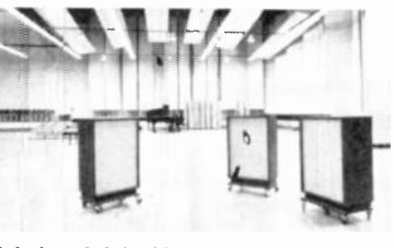
Interior of Columbia Records Studio (Hollywood) and Altec 605A "Duplex" loudspeakers used for PLAYBACK.
