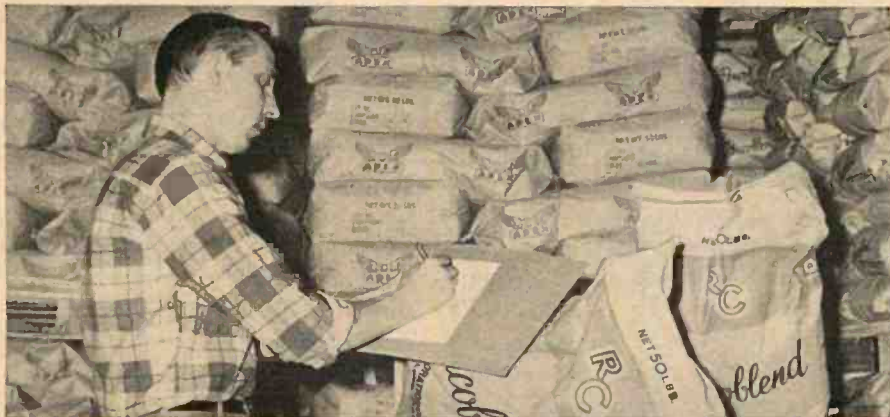
The receiving foreman at a record-manufacturing plant checks in fifty-pound bags of granulated vinyl. After being mixed with a plasticizer and carbon black, the compound is heated until it is about the consistency of putty; then it is molded into records.
