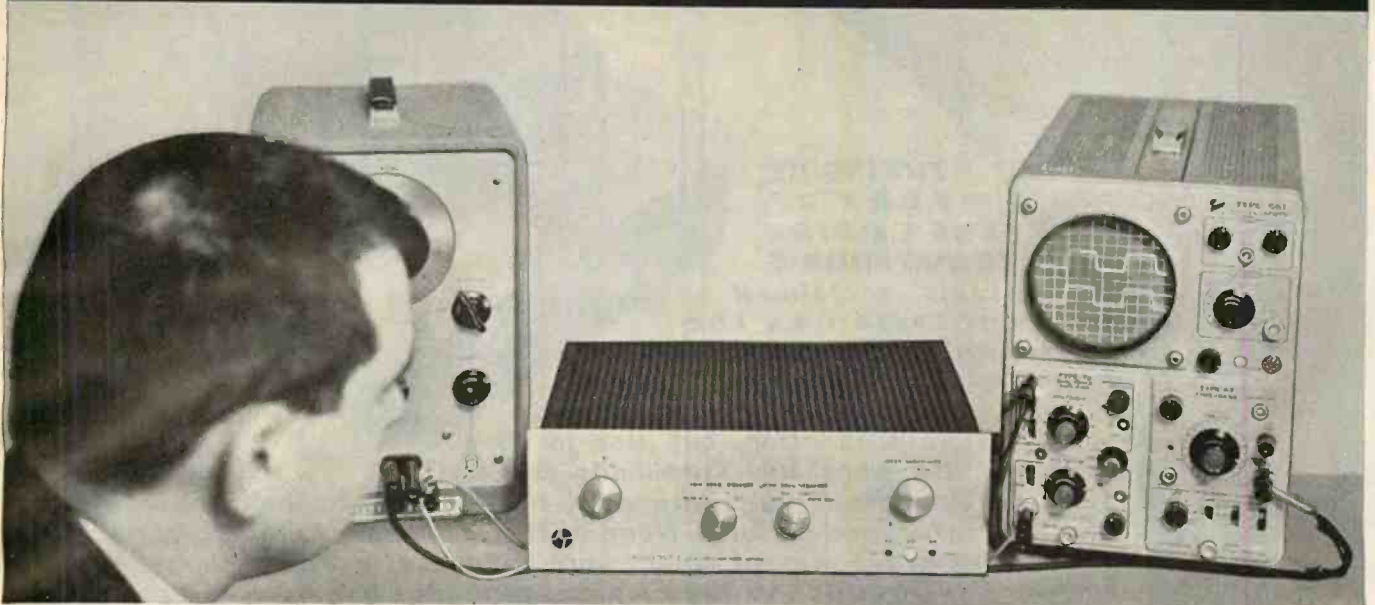
A fascinated audiophile at the 1962 New York hi-fi show observes the remarkable square wave response of the Acoustech I (the bottom pattern is the 20 KC output of the square wave generator . . . the top wave is the output from the Acoustech I).
