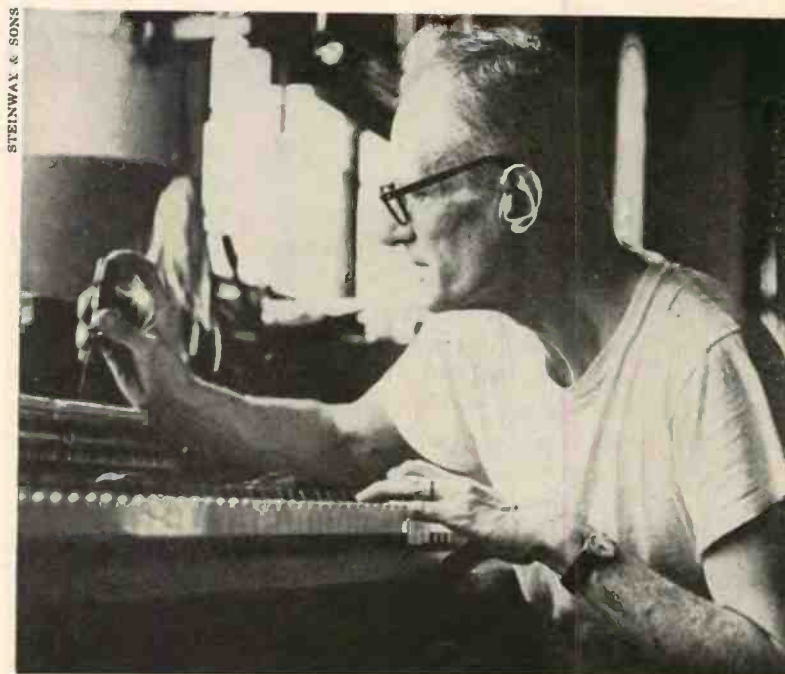
Regulating the action to obtain an even response from bass to treble is a job for a master craftsman.
