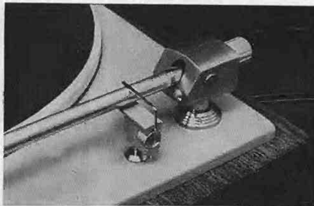
Bogen's arm moves in ball bearings, has spring tension adjustment, automatic arm positioner with safety latch.
