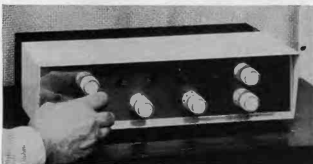
Lowest in cost among the stereo preamps tested in this article is the Arkay SP-6. Two-step rumble and scratch filters provide some channel tone control.
