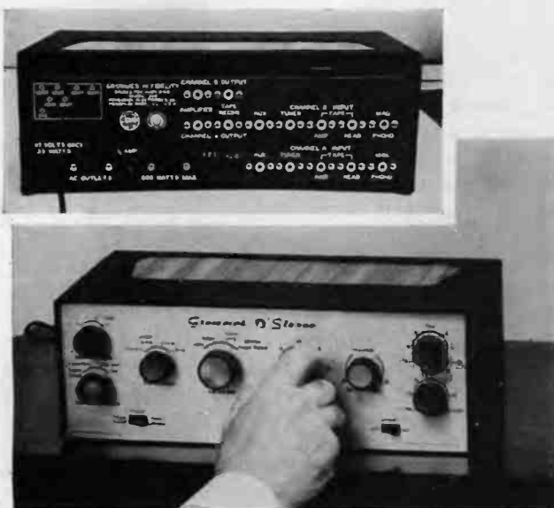
Prize winner for clean legible rear panel layout is the Grommes 208. Note how all phono input jacks are easily accessible and exceptionally well-marked.
