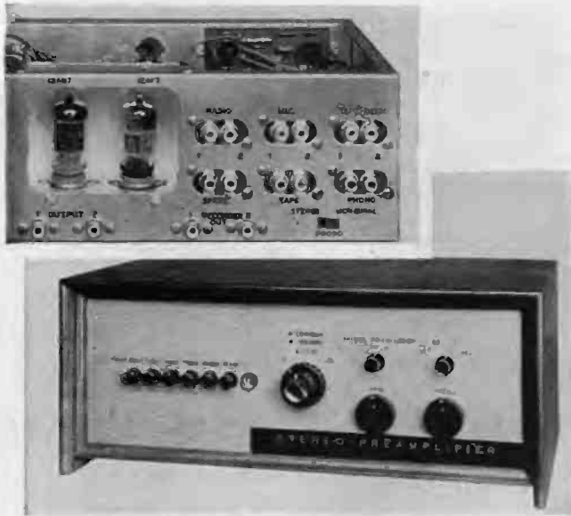
Altec Lansing utilizes four transistors visible on the printed-circuit panel. The two tubes mounted on the rear apron are the only heat-producing elements.
