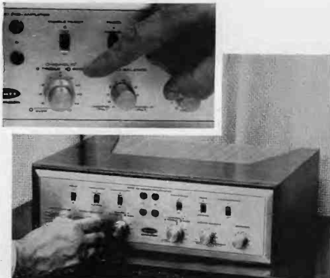
Individual tone controls on each channel are important features in the Scott 130. Switch above finger inverts phase of Channel B amplifier.
