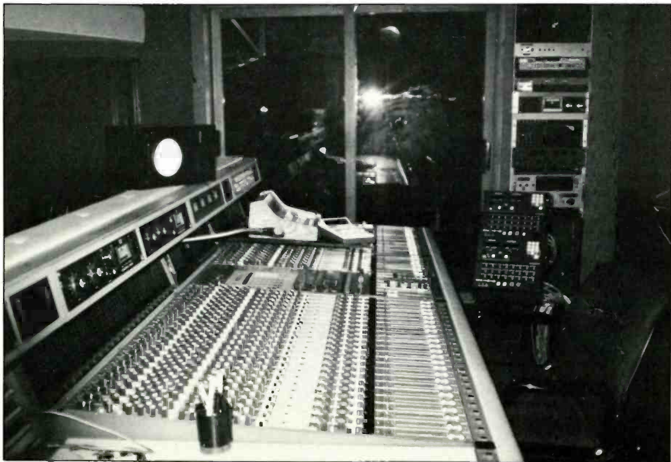
Figure 1. Neve 8128 48-channel recording console with Neve 1173 in Music 1, with equipment room off right.
