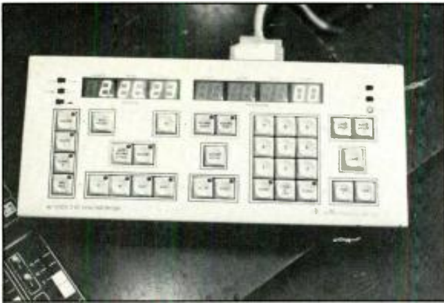
Figure 2. Close-up of operator's computer terminal/controller of Q-Lock 3.10.
