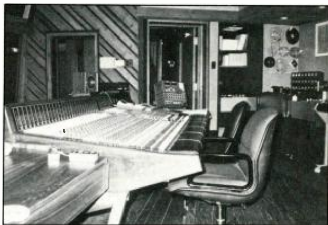
Figure 5. View from producer's desk of Harrison 4032 C transformerless console in Music II.
