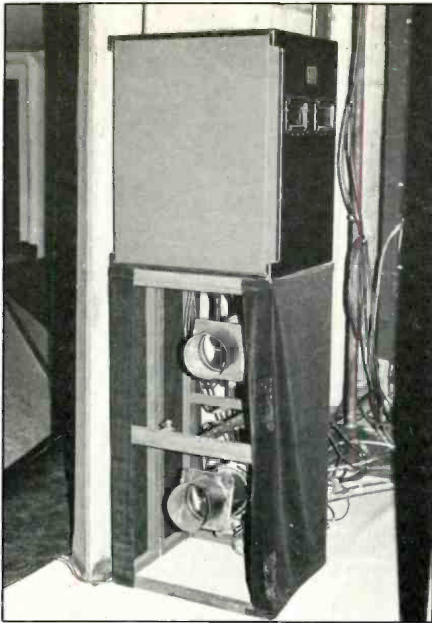
Figure 6. A-1 Audio custom JBL 4320 cabinet with Gauss 4580 and JBL 2441 compression driver and 2402 tweeter.
