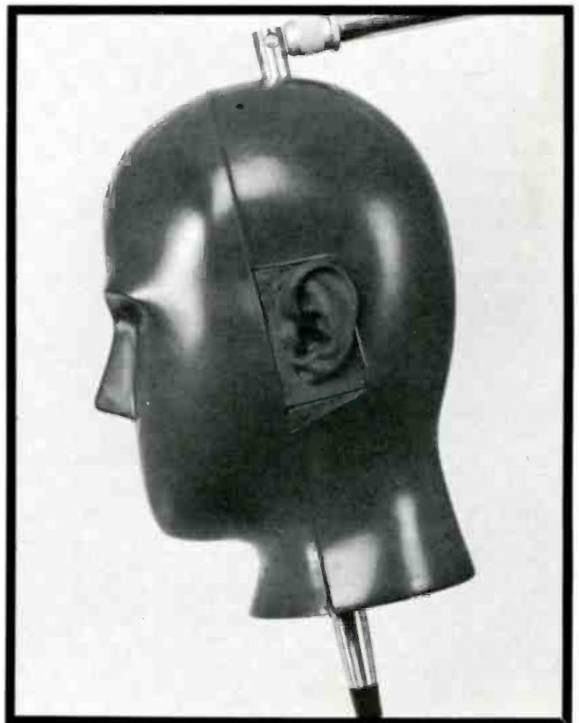
Figure 2. The diffuse field equalized artificial head: Recordings made with this head are also suitable for reproduction through loudspeakers.
