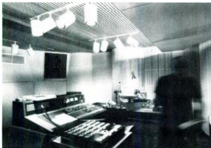
Front view of new mastering room with UREI speaker in place and cutting engineer George Piros flashing by at high speed. The cutting equipment is the Neumann VMS-70 system.
