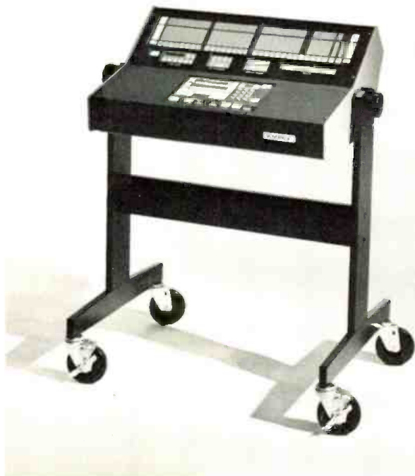
Figure 2. A roll-around pedestal containing the channel function and multi-point search-to-cue modules.
