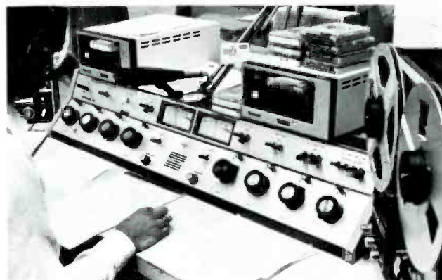
An operator's-eye view of the Harris Stereo 80 board, flanked by Revox and TEAC tape recorders.
