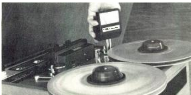
Reading dynamic tension on moving tape with a tension gauge.
