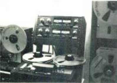
tari showed a rugged half-inch four track unit built around the basic 5050 Mark II series.
