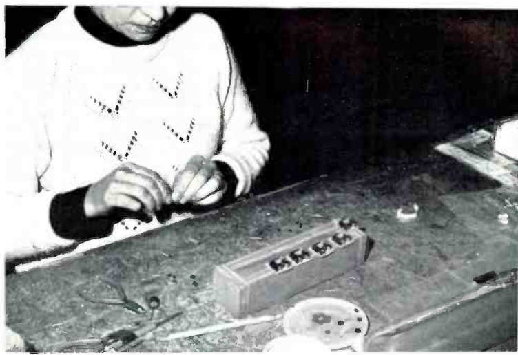
Audio Designs manufactures its own operational amplifiers, here shown at an intermediate stage of production.
