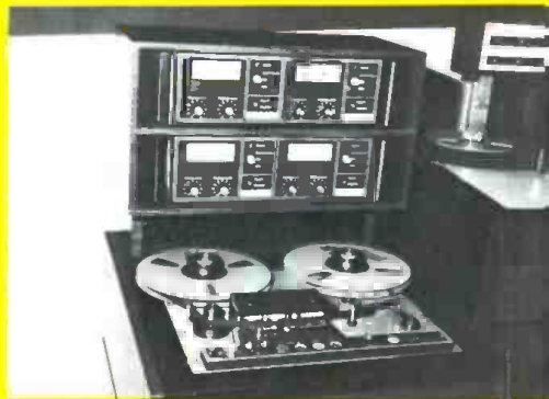
Dictaphone's newest recorder is the Scully 280-B four track model. Circle 51 on Reader Service Card.
