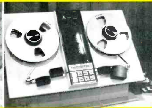
Recortec makes this bi-directional duplicating master which feeds a loader and slaves. Circle 99 on Reader Service Card.
