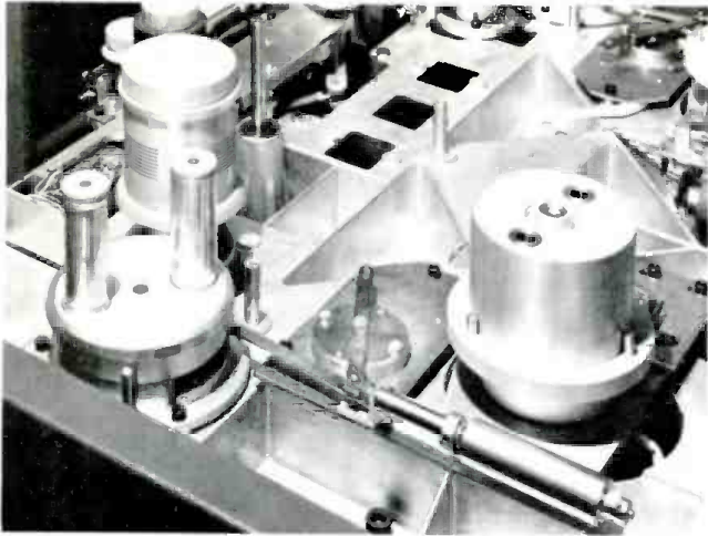
Two contact free sensors are provided for controlling the torque of the spooling motors. The one shown at the left of the above picture, is for the take-up motor. Each contains a precision potentiometer which keeps the servo input voltage proportional to tape tension. Behind the two slender rollers of the tape tension sensor is the larger rotating roller. Bottom right is the damping element and right center the large take up motor hub for the reel.
