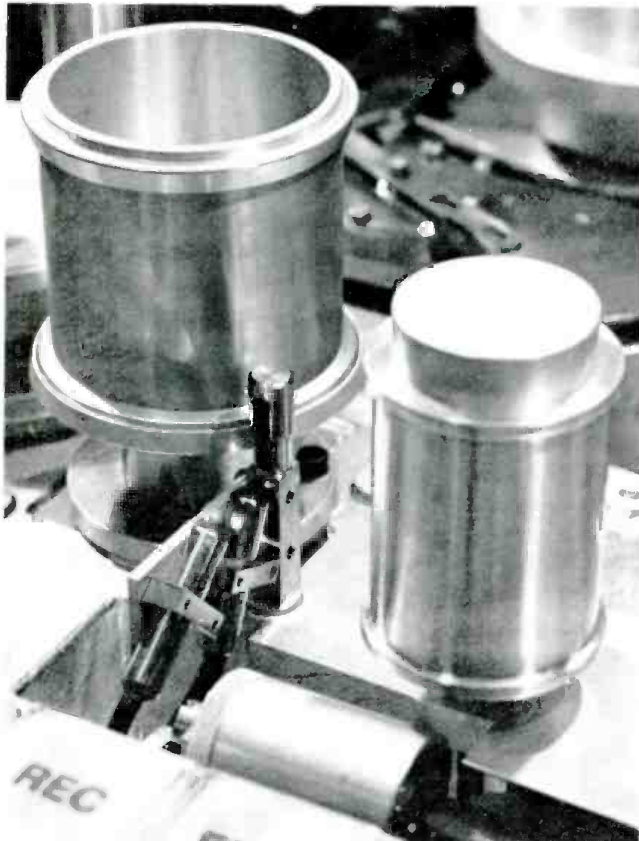
The photoelectric switch located next to the left rotating idler provides information regarding the presence or absence of tape. This element consists of a lamp with lens at bottom left, the photo-element in the second cylinder and a mirror system within the slender vertical column. Only in the absence of tape does the light reach the photo element via the mirror located behind the tape.
