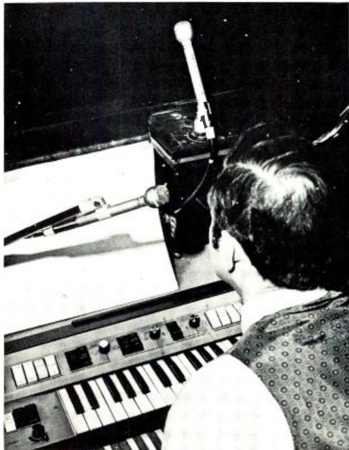
Figure 3. The mics used by the rock band singers are often only inches from the footlight stage mics. However, the directional characteristics of the mic (an E-V RE15) prevent leakage problems.
