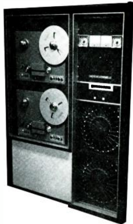
Figure 1. A commercial automation system with two reel machines, a single cartridge player, and two Carousels. This unit was built by Continental Electronics and is installed at KOL-FM, Seattle, Washington.
