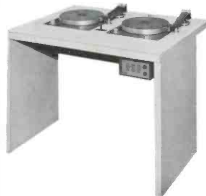
Figure 2. The turntable module used in the control room at KMOX. Note the cue amplifier below the right turntable.
