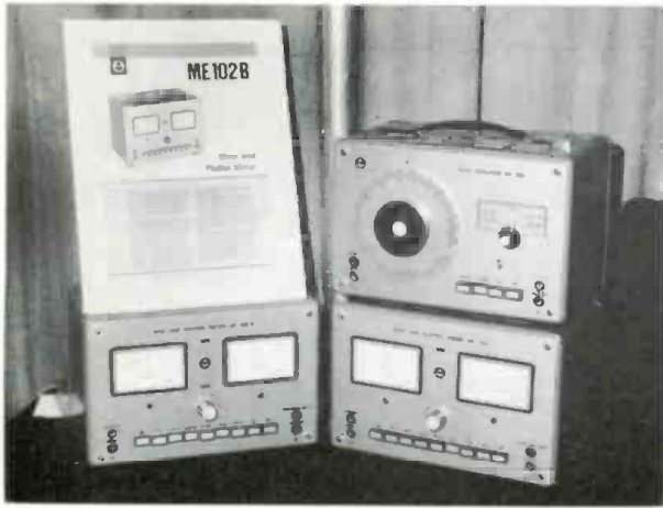
Gotham Audio ME102B, ME104 wow/flutter meters and ME301 wave analyzer. Circle 29 on Reader Service Card.
