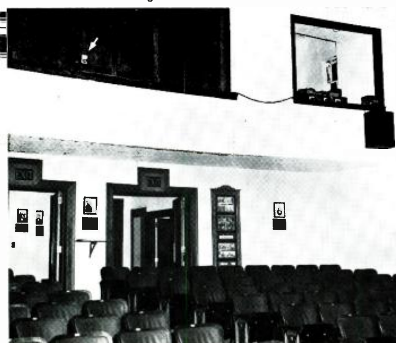
Fig. 1. An audience-eye view of the sound booth at The Players Club of Swarthmore. Note the rear theater speaker directly under the booth's window. A small tv camera is at the upper left. This pipes a picture backstage so that offstage personnel can see the stage action.
