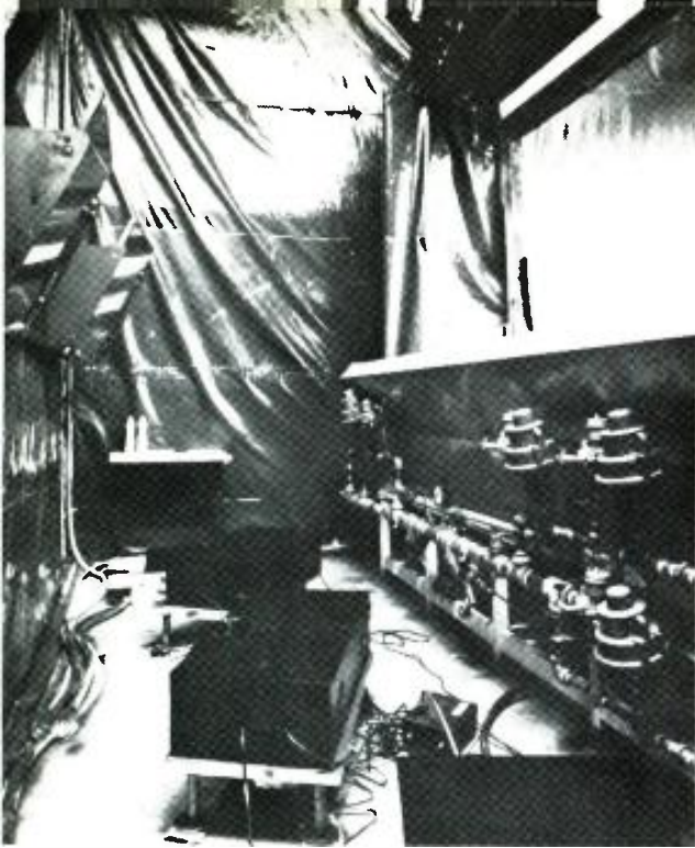
Fig. 7. This behind-the-scenes view at Kodak shows the set-up used for the water screen projection. The hydraulic system used to create the water screen extends from the right to the center. The black boxes in the foreground each contain a pair of projectors as seen in Fig. 6. Each is covered, but a cutout allows the image to be reflected by mirrors onto the wall mounted mirrors (upper left), then to the water screen.
