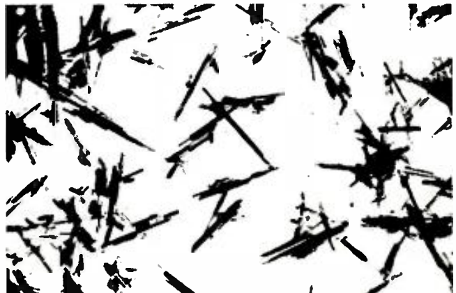
Fig. 1. This electron photomicrograph of chromium dioxide crystals at 50,000 times magnification illustrates the uniform, needle-like particles which permit better orientation.
