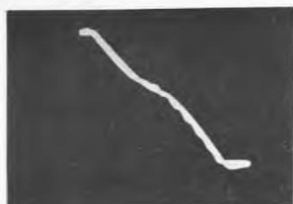
1-Kc input-output Lissajous trace at 20% overload through power amplifier only.
