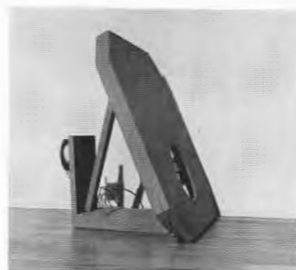
Fig. 1. Mounting board for midrange speaker and filter built by the author.
