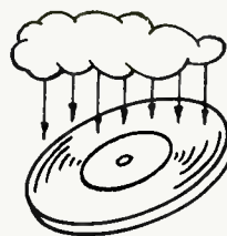
DISC IS COATED WITH SILVER TO MAKE METAL "MOTHER"
