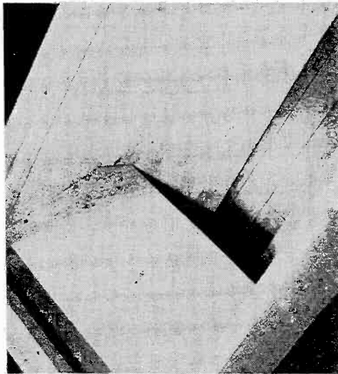
Fig. 4. It may take some effort to get lower horn-shaping piece firmly against back panels and short side-panel cleats.
