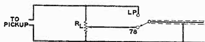
Fig. 1. Arrangement to get equal output of pickup cartridge on 78's and LP's.
