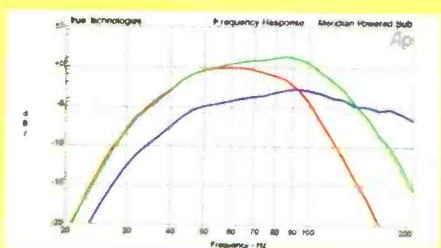
Fig. 4—Frequency response, M1500 subwoofer, low-pass filter set flat (blue), at 120 Hz (green), and at 80 Hz (red).
