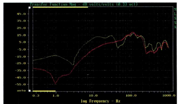
FIG. 2 —Response of “TH 4-15” system. This is another infinite baffle design, using four 15-inch drivers, in a rectangular room approximately 2,200 cubic feet in volume and with just one, large open doorway. Heavy curve is near-field, the faint curve room response at 3 meters. Maximum room reinforcement is about 17 dB at 5 Hz.
