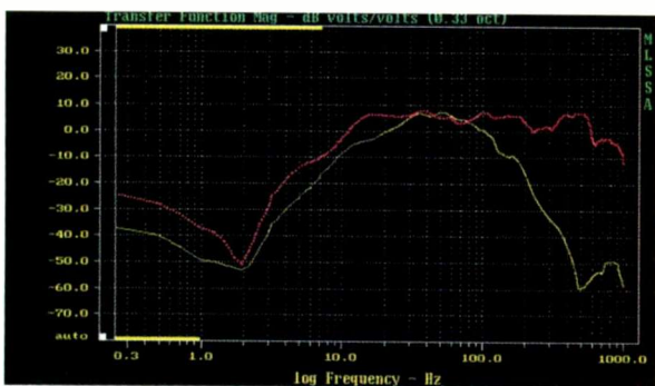
FIG. 4 —The “TP 8-12” is an infinite baffle system with eight 12-inch drivers built into an attic eave. The room is a loft. The main listening area is about 2,450 cubic feet, but the back opens into a two-story space that makes the total volume about 8,000 cubic feet. The heavy curve is a near-field measurement, the faint one a 3-meter room response. Room reinforcement begins at 30 Hz and reaches a maximum of approximately 12 dB.
