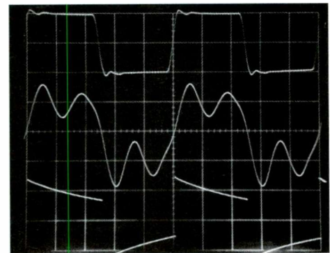
Fig. 2—Square-wave response of Triode 100 SB for 10 kHz into 8 ohms load (top), 10 kHz into 8 ohms paralleled by 2 \mu F (middle), and 40 Hz into 8 ohms (bottom); all tests made at 8-ohm tap.
