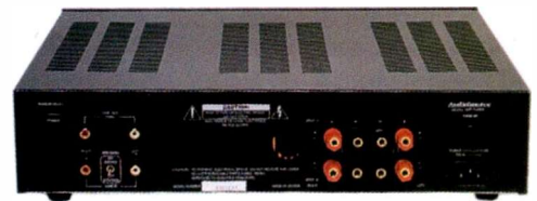
A switch on the AMP Three's rear panel enables automatic power-up from standby mode.
