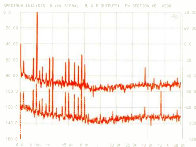
Fig. 6—Spectrum analysis, FM stereo mode, one channel modulated with 5 kHz (solid curve), other channel unmodulated (dashed curve). Use the right-hand scale for the lower curve.
