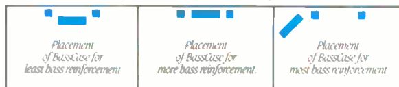
Bass frequencies are essentially non-directional, so you can place BassCase where it sounds best in the room. The mid and high frequencies, and the stereo effect are reproduced by a pair of small "satellite" speakers.
