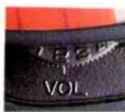
Dual volume controls permit right and left channel adjustment.
