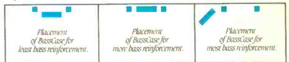
Bass frequencies are essentially non-directional, so you can place BassCase where it sounds best in the room. The mid and high frequencies, and the stereo effect are reproduced by a pair of small "satellite" speakers.
