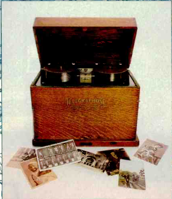
Wire recorders, the earliest actualized form of magnetic recording, were shown in Smith's drawings. This American Telegraphone, which belongs to recording historian Bob Angus, was foreshadowed by Smith's ideas.
