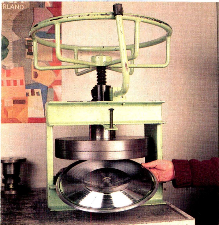
The last step before mounting the stamper in the record press is to form its shape so that the proper record profile will then be pressed.
