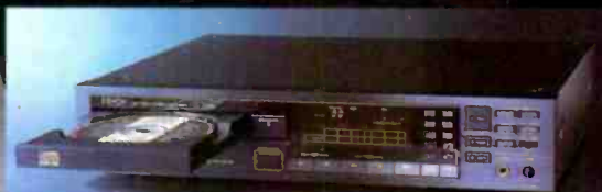
DCD-1500: Dual Super Linear Converters; Oversampling Digital Filters; CALP Analog Filters; Programming; Remote Control.
