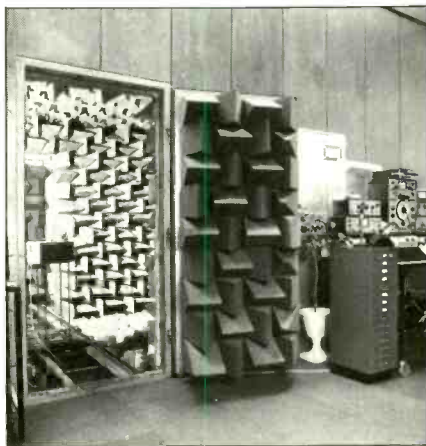
Anechoic chamber and test instruments in Steyning research establishment
