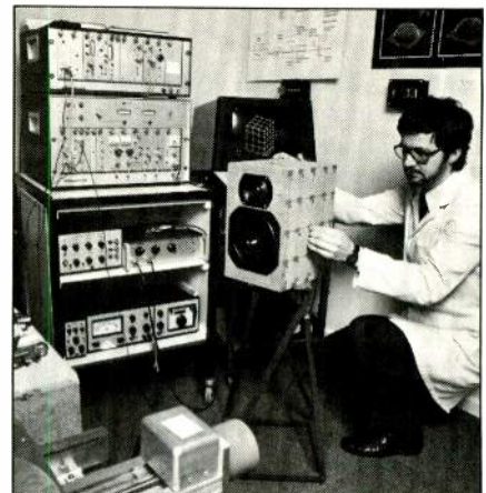
G. J. Adams setting up laser interferometer test of cabinet resonance
