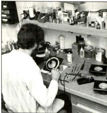
Constructing drivers used in the B & W Modular Automobile Sound System
