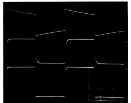
Fig. 5— Preamp line-amp square-wave responses for 20 Hz (top), 20 kHz (middle), and 20 kHz at clipping (bottom).
