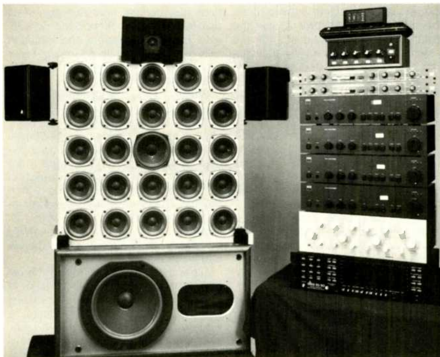
Fig. 9—An early prototype of the MGC-1, which had a directional array.
