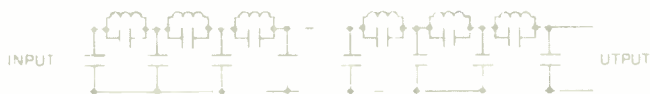
Fig. 2—A passive, low-pass Chebyshev filter, showing cascaded design. The filter's "order" is the number of cascaded stages.
