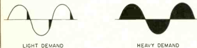
Fig. 1—With light demand, Phase Control Regulation delivers power-supply voltage only for a portion of each a.c. cycle; with heavy demand, the entire cycle is used.
