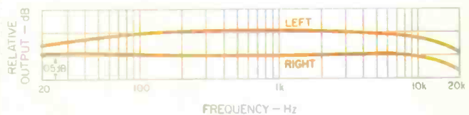
Fig. 2—Phono EQ error with IHF load at tape out, SP-10 preamplifier.
