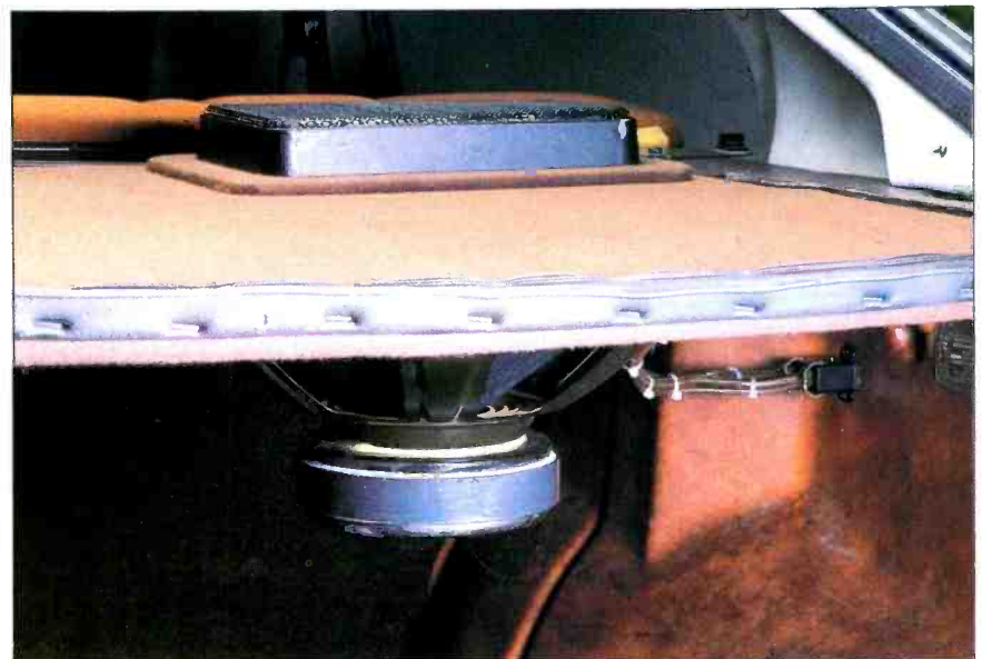
A new rear deck holds a pair of Genesis AM-165 speakers where they belong, at the front of the deck; dual 10-inch subwoofers are concealed beneath the cloth.
