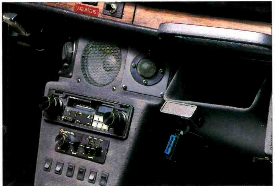
The new center console was chiefly built to hold the center speakers (see text). Note also the "bucket" beneath the dash at right, to hold equipment under test.
