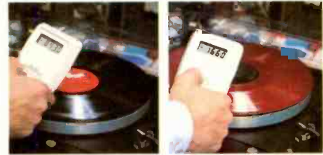
Strict record pressing standards, and audio and visual inspection, assure high quality. Ordinary records (left) have static charges that attract dust, causing surface noise. But the special anti-static vinyl used in Franklin Mint records (right) assures clearer sound. Electrostatic meter tests show that the Franklin Mint record has only one-fifth the static charge of ordinary records.
