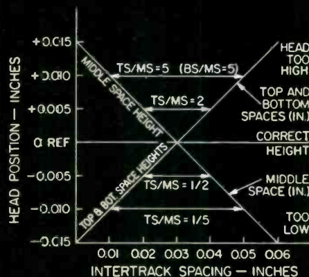
Fig. 9—Intertrack spacing as a function of vertical head position.
