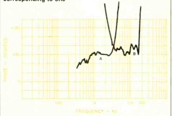
Fig. 4—One-meter anechoic phase response corrected for air-path delay of (A) 3.5053 mS and (B) 3.1742 mS.
