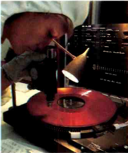
Franklin Mint proof-quality records are pressed in a dust-free, atmosphere-controlled "clean room," where careful methods of production and inspection assure the high quality of these great recordings.
