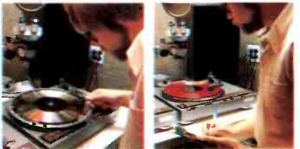
(left) You normally can't tell if the record you buy was the first or last to come from a record stamper, or if the stamper was made from a defective metal mold. But (right) The Franklin Mint Record Society aurally auditions a greater number of pressings than most other producers. And every metal mold is actually played, from start to finish, before it is used to produce stampers.
