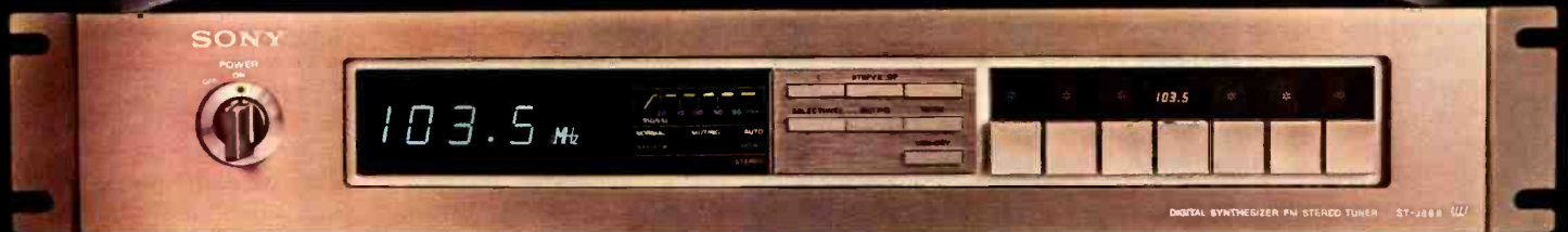
ST-J88B TUNER: Quartz lock frequency synthesis tuner / Varactor diode-MOS FET front end, with Uni-Phase IF filters / Auto and manual 'step' tuning or full 8-station memory with nonvolatile Sony MNOS memory IC / 2 discrete IF circuits for narrow and normal modes.
