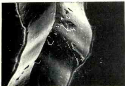
Fig. 6—SEM microphotographs of a recording of Rachmaninoff's Symphony No. 1 .
