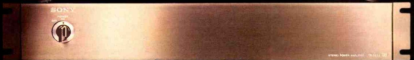
TA-N88B AMPLIFIER: Pulse Width Modulation (Class D) amplifier design / Vertical FET (V-FET) power output transistors / High regulation Pulse Locked Power Supply (PLPS) / 'Dual mono' amplifier configuration / 3-stage protection circuitry.
