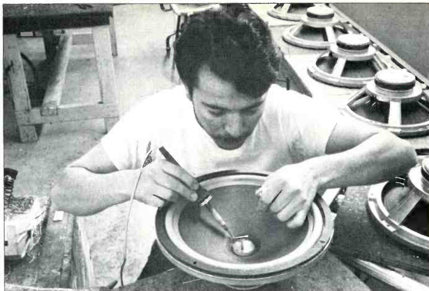
Production of loudspeakers at Cerwin-Vega's plant in Arleta, Calif.
