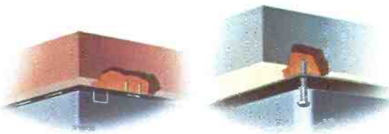
Common staples can work themselves loose, which is why Pioneer uses aluminum screws to mount the base plate to the base.
