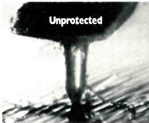
Magnification shows the record vinyl wearing away.
