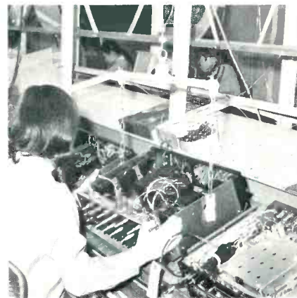
Assembly line at the Sansui operation showing the lifting cradle.
